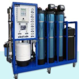
AMPAC USA offers Fully Packaged Reverse Osmosis Systems designed to fit end user application, those RO Systems include feed pumps, pre-treatment necessary as per end user water quality analysis reports, RO Process, and finally all post-treatment including post-filtration and Ultra Violet to guarantee best water quality at the point of use. The series ranges from 1500 GPD to 10,000 GPD
